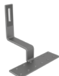
Art. 093 Pantile Roof Hook Standard Plate: 180x50x4, (12x)Hole: Ø7mm Bar: 30x5, long Hole: 9x47 Use: pantile roof Material: A2 1.4301 stainless steel, shot blasting
